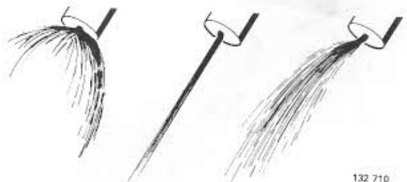
Examples of poor spray patterns (Injector should be replaced).
